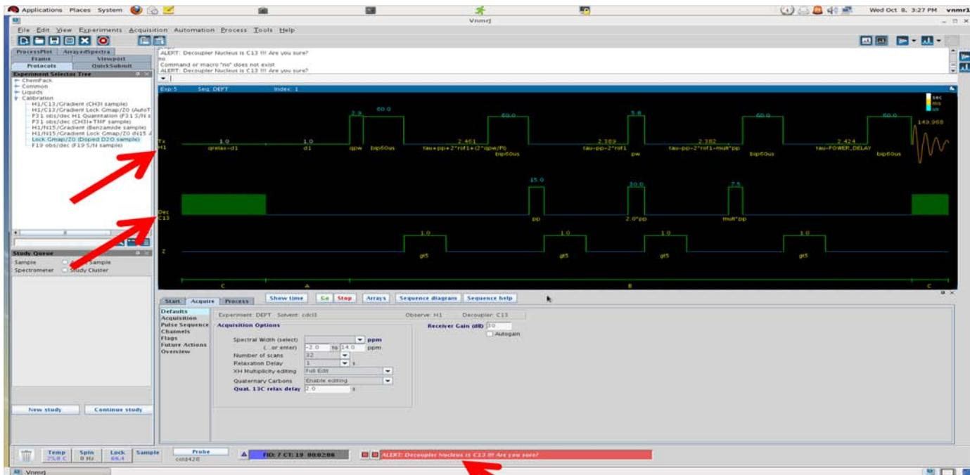
Also, the pulse sequence shows that the experiment will detect H1 and that the decoupler channel is set to  $^{13}\text{C}$ . This is wrong!
