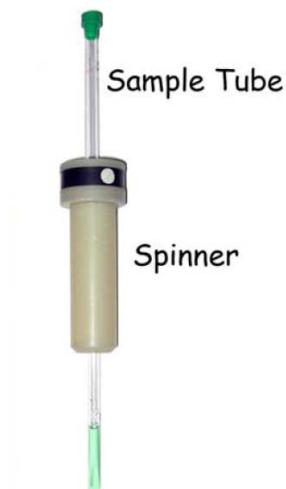
4) On the VNMRJ, type “e” and then press <enter>. Put the sample on top of the magnet. Type “i”/<enter> to insert the sample in the magnet.
