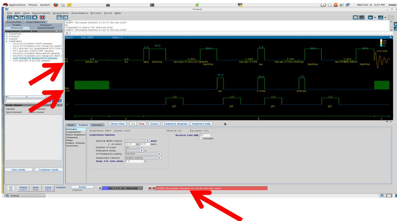
Also, the pulse sequence shows that the experiment will detect H1 and that the decoupler channel is set to  $^{13}\text{C}$ . This is wrong!
